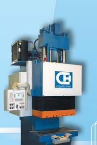
HSP 160 \* 5 \* XC 1600 kN press with CNC press control
