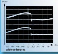
Oscillograh Blanking operation on a 12000 kN hydraulic press, blanking force 9500 kN, material thickness 22 mm St 00.
