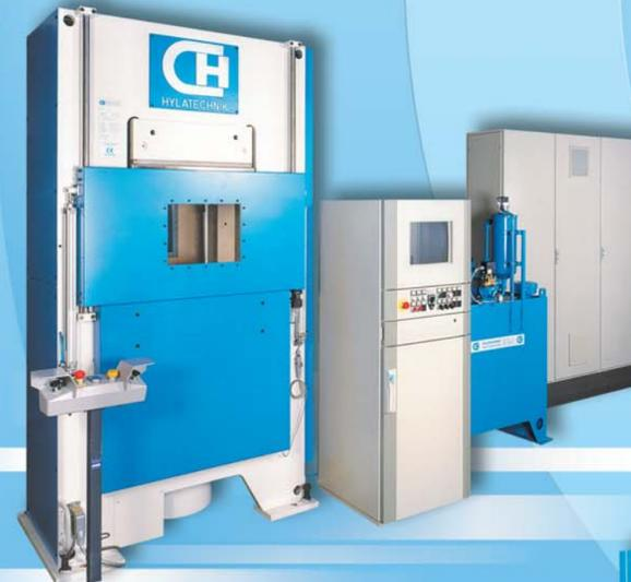
2000 kN sinter press with
